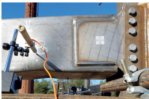
Photo 4. Deformation scheme of the lap joint type socket of suspension pole (I-GP-1)
