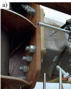
Photo 5. Deformation scheme of the head joint type socket of tension pole (II-GM-2): a) compression zone, b) tension zone
