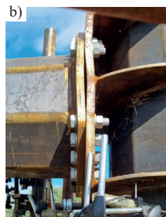
Photo 5. Deformation scheme of the head joint type socket of tension pole (II-GM-2): a) compression zone, b) tension zone
