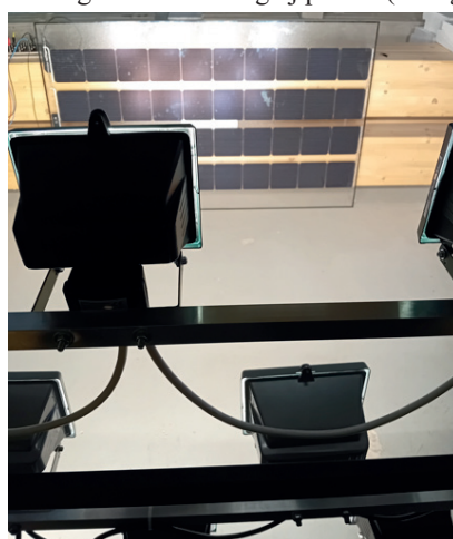
Photo 4. Measurement of the operational electrical properties between panel loading cycles
