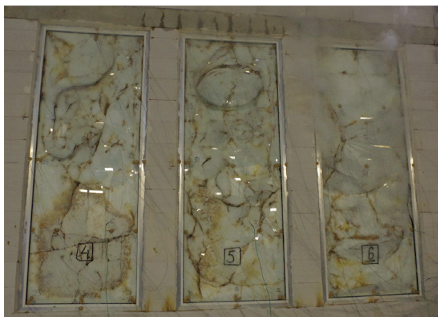
Photo 3. The test specimens with IGUs with 8 mm spacers frame in 68 th minute of the test
