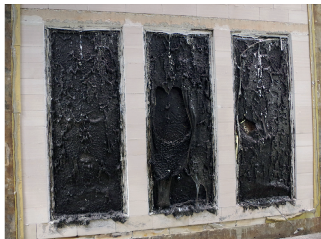
Photo 7. The exposed surface of test specimens with IGUs with 14 mm spacers frame after the test
