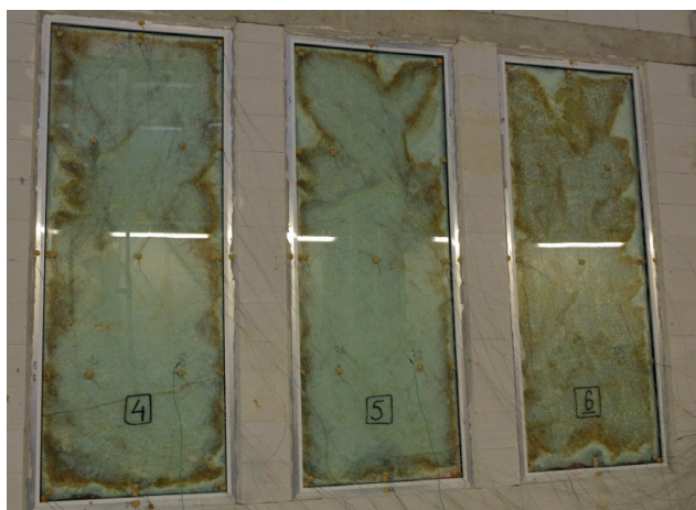
Photo 2. The test specimens with IGUs with 8 mm spacers frame in 5 th minute of the test
