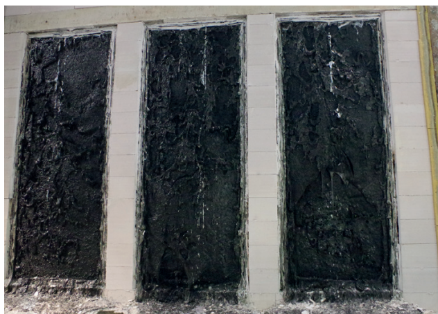
Photo 6. The exposed surface of test specimens with IGUs with 8 mm spacers frame after the test
