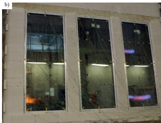
Photo 1. Test specimens in the first minute of the fire resistance tests: a) IGU with 8 mm spacer frame and VSG 33.2 glass; b) IGU with 14 mm spacer frame and VSG 33.2 glass
