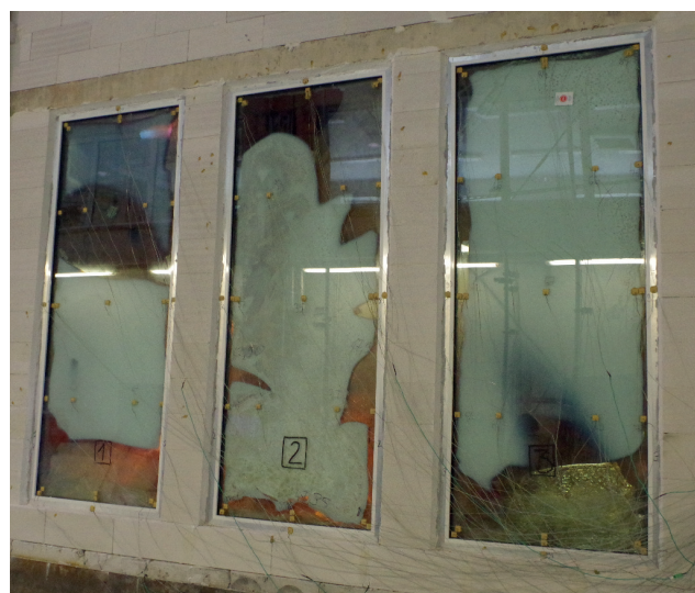
Photo 4. The test specimens with IGUs with 14 mm spacers frame in 5 th minute of the test
