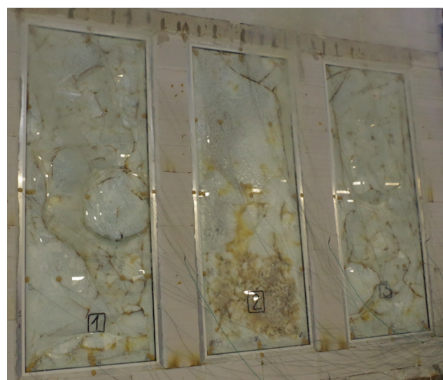
Photo 5. The test specimens with IGUs with 14 mm spacers frame in 68 th minute of the test
