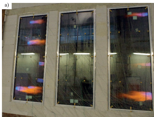
Photo 1. Test specimens in the first minute of the fire resistance tests: a) IGU with 8 mm spacer frame and VSG 33.2 glass; b) IGU with 14 mm spacer frame and VSG 33.2 glass
