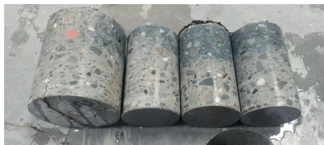
Photo 5. Example view of drill cut samples from the floor, crack extending over entire floor slab cross-section (location 2), evident colour variation visible on cross-section
