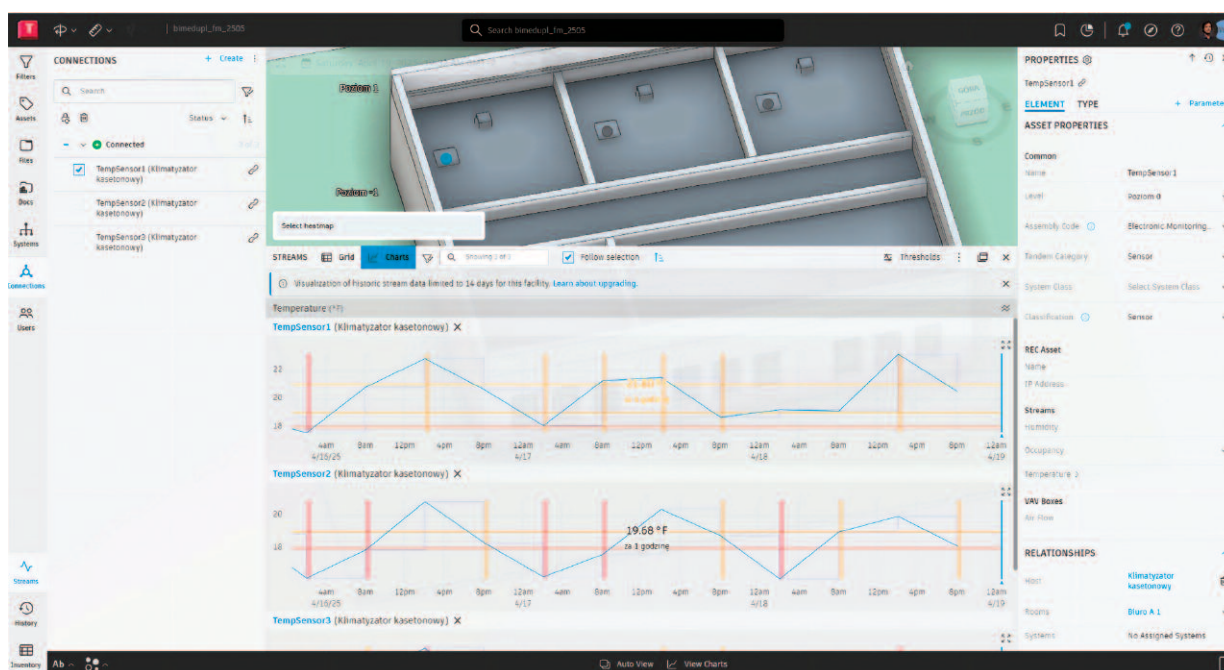
Fig. 6. Diagrams of temperature sensors continuously transmitting data from the building to the model
