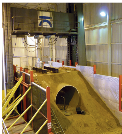
“STEND” test stand with a built-in GRP culvert
