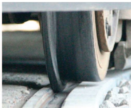
Photo 4. Due to the lack of narrowing of the rail groove acting as a guard rail for the right-hand wheel, the rim of the left-hand wheel hits the nose of the frog
