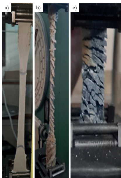
Photo 6. Tensile tests: a) sample no. 3, without changes in polyurea properties; b) and c) samples from below the wastewater surface, with clear signs of damage to the polyurea structure
