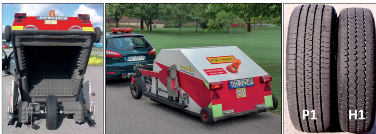
Photo 4. CPX test trailer and two reference tyres P1 and H1 [7]
