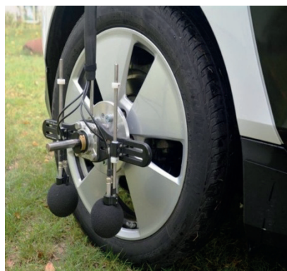
Photo 5. Tests of noisiness of the pavement using the OBSI method [8]
