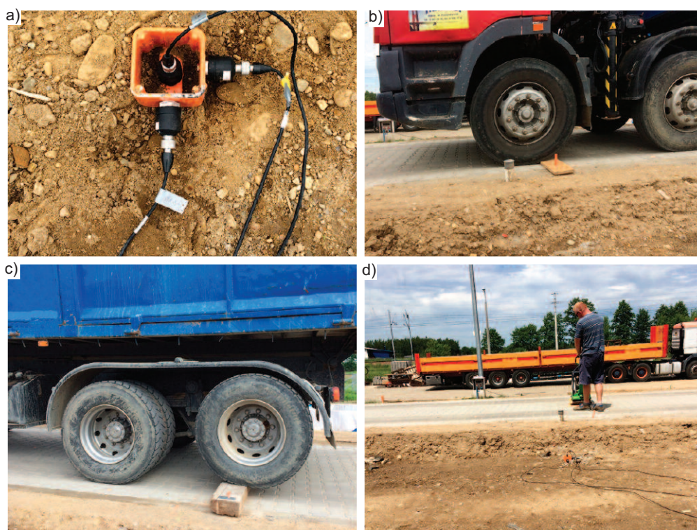
Photo 3. Acceleration sensors installed in the steel base (a); passing over a low threshold (b); descending from a high threshold (c); forced by construction compactor (d)
