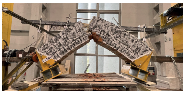
Photo 3. Collapse moment of the FRCM-reinforced compress arch (RCA)
