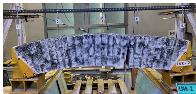
Photo 4. Collapse moment of the unreinforced tensioned arch (UTA)
