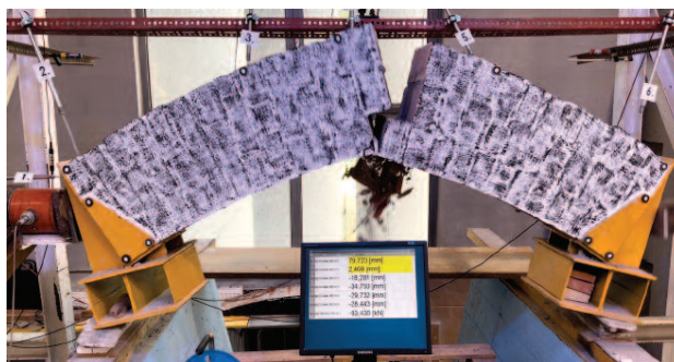
Photo 2. Moment of failure of the unreinforced arch (LNS)
