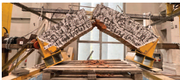
Photo 4. Moment of failure of the arch reinforced with FRCM technology (LWS)
