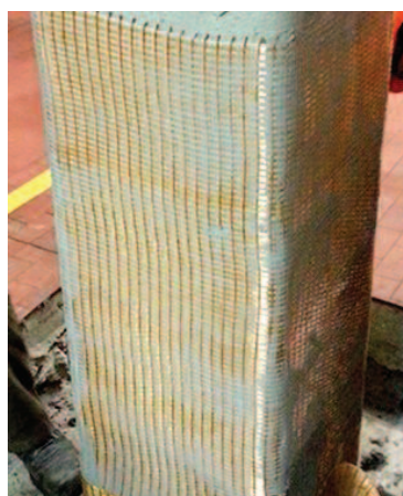
Photo 1. Example of the application of PBO-FRCM composite – eccentric compression strengthening [2]
