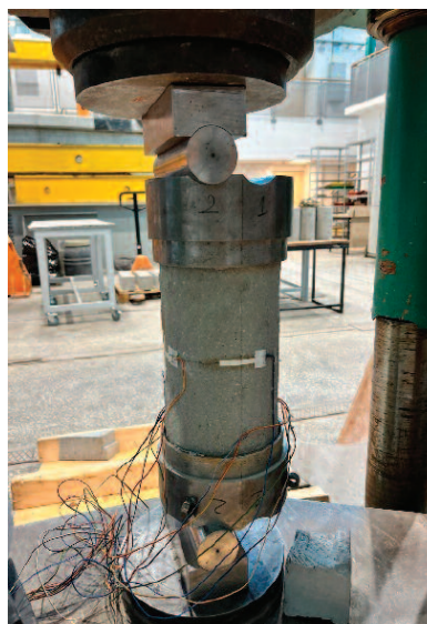
Photo 3. Steel plates with hinges for eccentric loading
