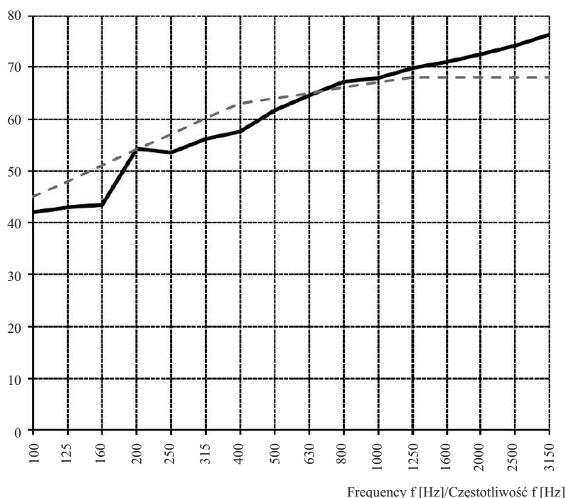
Fig. 3. Measured sound insulation as a function of frequency for the ceiling between the garage and the apartment above
