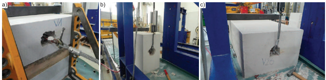
Photo 3. Testing the transport anchor in the longitudinal direction (a); perpendicular to the thickness (b) and perpendicular to the width of the element (c)
