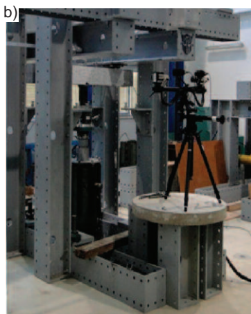
Photo 1. Stand for shear capacity testing of bend elements: a) beam side surface tested using SAD-256 system; b) beam side surface tested using Aramis 4M system
