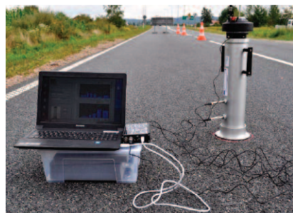
Photo 1. Spectronics ACUPAVE System – measurement on the road surface Fot. 1. Spectronics ACUPAVE System – pomiar na nawierzchni drogowej
