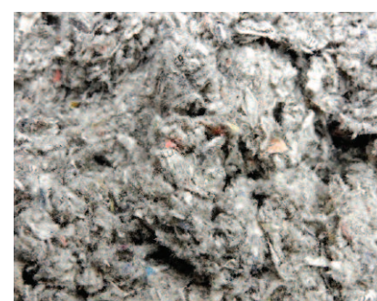
Photo 2. Cellulose sample prepared by blowing the material into the test mold – a homogeneous mixture fills the entire empty space
