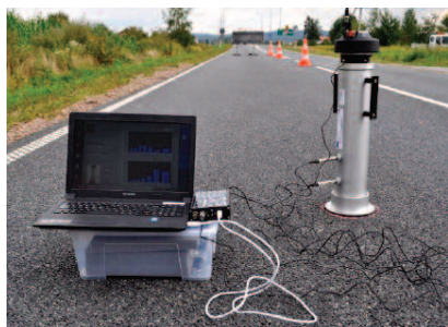
Fot. 1. Spectronics ACUPAVE System – pomiar na nawierzchni drogowej Photo 1. Spectronics ACUPAVE System – measurement on the road surface
