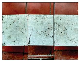
Photo 2. The course of cracks in B0 samples subjected to compressive strength testing. Failure pattern typical of high-strength concrete
