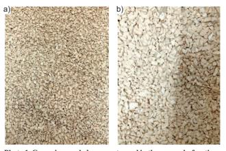
Photo 1. Ceramic recycled aggregate used in the research; fraction: a) 4-8 mm; b) 8-16 mm
