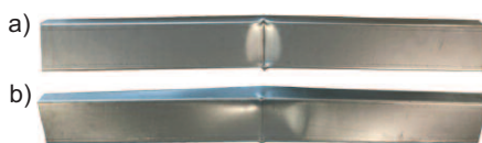
Fig. 7. The tested cold-formed steel beams: a) without stiffening; b) with stiffening in the form of an insert made in 3D printing technology
