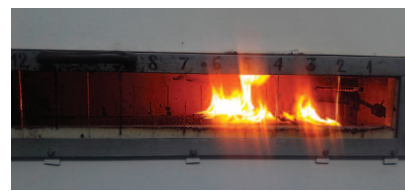
Fot 3. Widok próbki podczas badań wg PN-EN ISO 9239-1:2010 [Fot. Autor] Photo 3. View of the sample during tests according to PN-EN ISO 9239-1:2010
