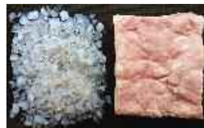
Photo 1. Aerogel granules (left) and aerogel-enhanced blankets obtained embedding a fiberglass panel with precursor aerogel before the drying process (right); both created at Ryerson University
